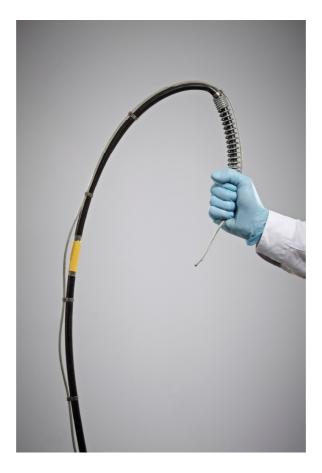
Image shows that although the assembly has been subjected to excessive loading and has thus surpassed its minimum bend radius, the mechanical join between the ferrule and hose is protected by
